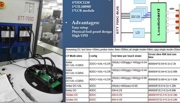
Wafer Test Solution -- multisite AC+DC test
