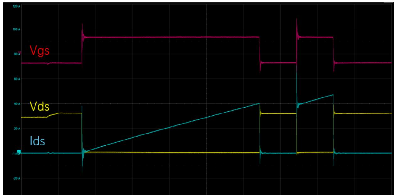
above is a SiC Mosfet double pulse switching test waveform, some parameters like  $T_{don}=15.2\text{ns}$ ,  $T_{rr}=61.4\text{ns}$
