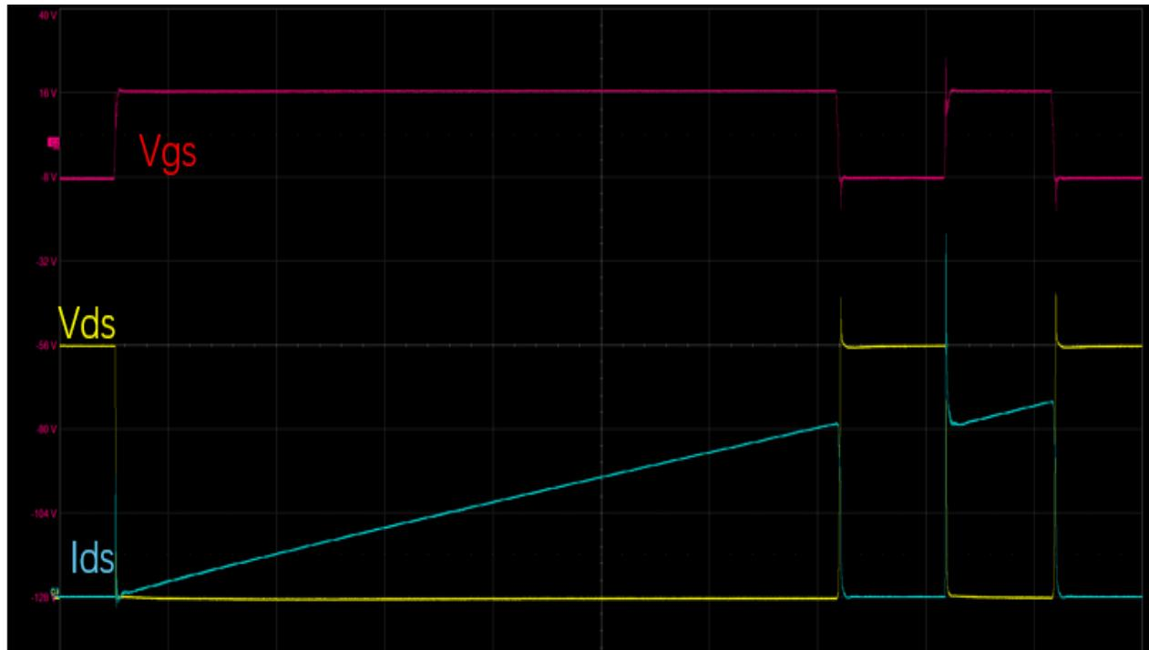
above is an IGBT double pulse switching test waveform, some parameters like  $T_{don}=12.7\text{ns}$ ,  $T_{rr}=259.9\text{ns}$
